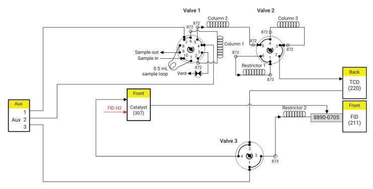
Figure 1. Gas chromatograph plumbing diagram.
