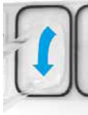
Figure 6. Drag and dispense method – Start dispensing when the pipette tip is near the top of the well. Finish dispensing when the pipette tip is near the bottom of the well.
