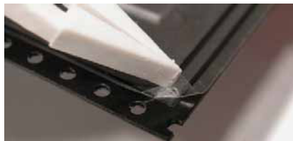
Figure 2. Removal of clear plastic covering
