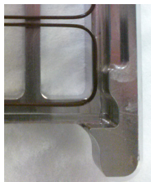
Figure 7. Correct positioning of gasket slide in chamber base
